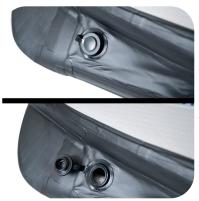
Side drains are intended to drain accumulated water while ashore. Leaving the drains opened while on the water will cause water to enter the kayak. Keep drains closed while kayak is in use. If drains leak, refer to Troubleshooting.
