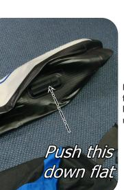
Fold one wall over the other. Push the floor in between the walls for a tight, compact fold.
